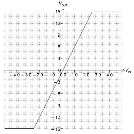
general shape of graph correct; straight line between –2.5 V and 2.5 V; plateau at –15 V and +15 V beyond this;
