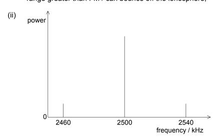
central band drawn at correct position; shorter side bands at correct positions;
